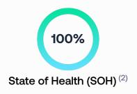
Remaining usable capacity / Usable capacity when new<sup>(3)</sup>
