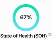
Remaining usable capacity / Usable capacity when new (3) 20.1 kWh / 30 kWh BMS reset (4)
